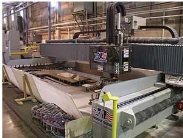
The fabrication facility also houses two Northwood CNC stoneworking centers.
