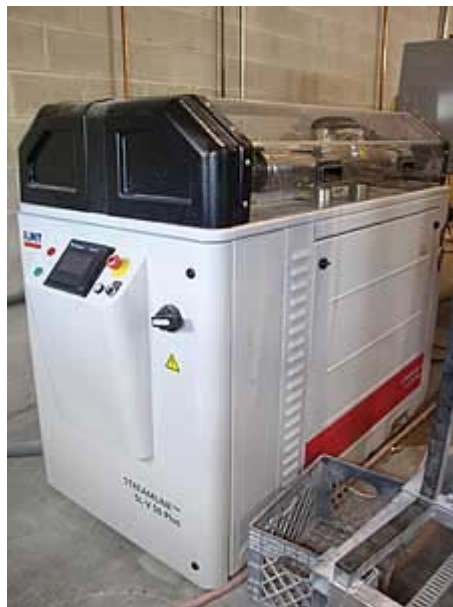
The SawJet is equipped with a Streamline™ SL-V50 Plus pump from KMT Waterjet Systems of Baxter Springs, KS.
