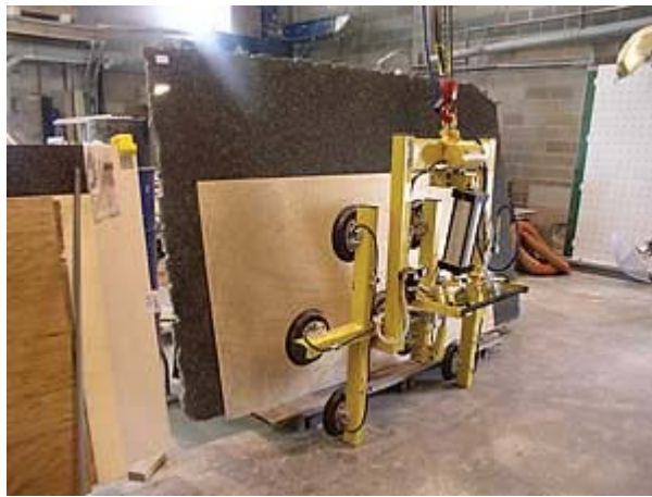
Slabs are lifted with vacuum lifters from Wood's Powr-Grip of Laurel, MT.
