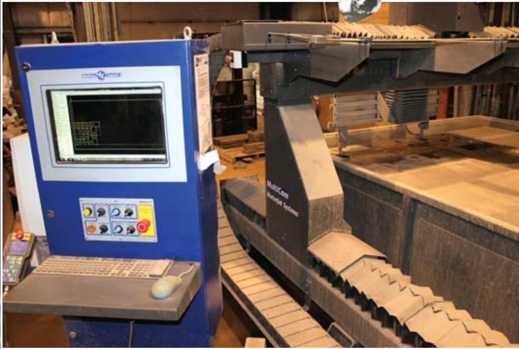
The MultiCam waterjet cutting system with KMT's 90,000 psi pump is helping Alco cut better quality materials at faster rates.
